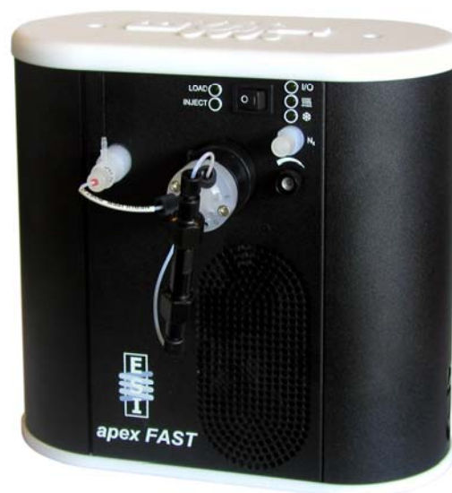
Apex-FAST with injection loop replaced with pre-concentration micro-column
