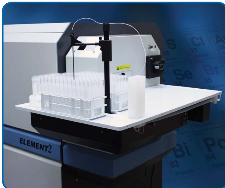
SC-E2 DXS integrated on the Thermo ELEMENT 2 ICPMS with integrated MP 2 micro peristaltic pump
