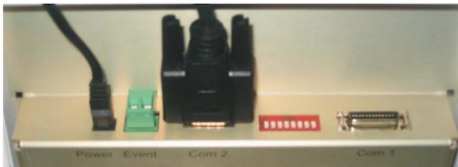
**Figure 6: AS-93+ Connections & Switch.**
