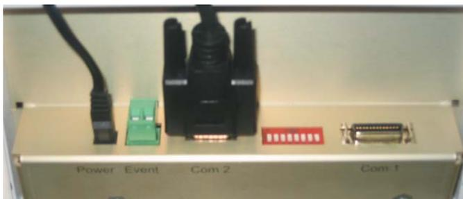
**Figure 2: AS-93+ Connections & Switch.**
