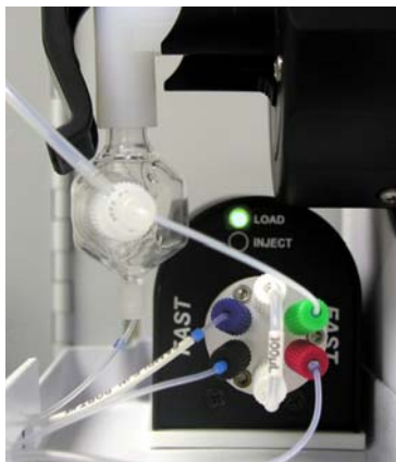
Injection Valve, PFA Nebulizer & Cyclonic MiniChamber
