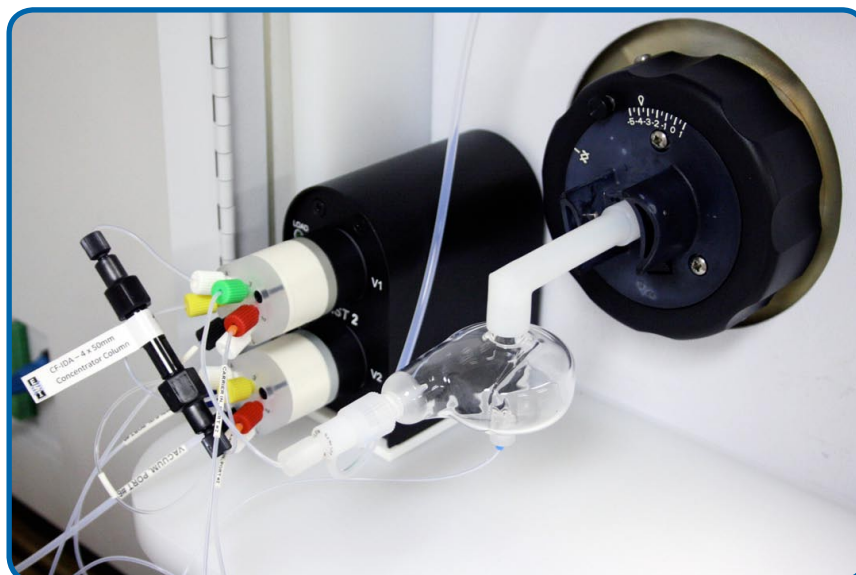
Figure 1. Close-up brineFAST valve system/PE Optima for automated determinations of Ca, Mg, Fe, Mn, Sr, Ba, Ti in 30% NaCl Brine.
