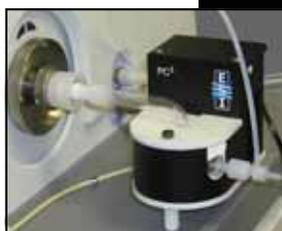
The PC3 can be adapted to a wide variety of ICP injectors, including ESI PFA injector base and quartz ball joint injector. The PC3 shown here is connected to the ELAN injector normally used with the PE Ryton spray chamber.
