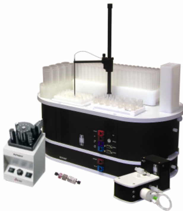
SC-FAST used in combination with Hg-C micro column and peristaltic pump to separate Hg species.
